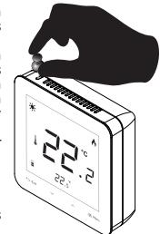
Holding the registration button on the controller for a few seconds will enable synchronization and consequently any change in the pre-set temperature in the main controller will automatically result in the same change in the regulator. Without synchronization, a change in the pre-set temperature in the main controller will cause a change in the regulator after a momentary delay.
