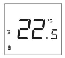
• **Hysteresis** - underfloor heating hysteresis defines the tolerance for the maximum and minimum temperature. The settings range is from 0,2°C to 5 °C.
