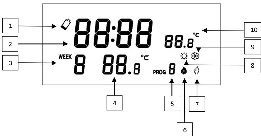
1. Low Battery Icon – Displays when the battery voltage drops below a certain level. Replace the batteries as soon as possible.
