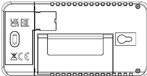
To insert/replace the battery, pull out the regulator cover as fully as possible.
